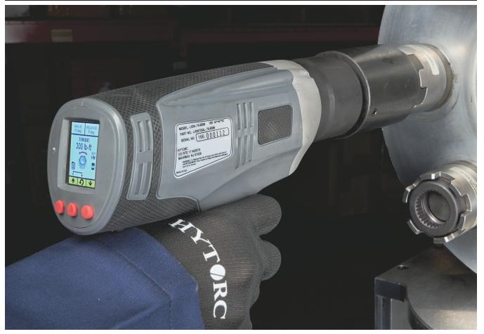
NOTE: The HYTORC Nut inner sleeve is tightened in the counter clockwise direction (left hand threads).
