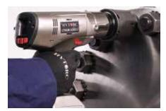
A direct torque measurement system utilizing a strain based transducer in a closed loop monitoring system provides more repeatable torque and enables advanced bolting features.
