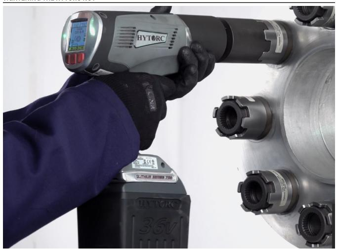
NOTE: The HYTORC Nut inner sleeve is tightened in a counter clockwise direction (left hand threads).
