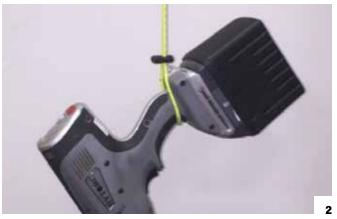
The LITHIUM SERIES Tool is a rugged industrial tool with an electric motor and electronic control. The following environmental considerations will help maintain reliable tool operation. Pictured above, keep cooling vents clear (1), and secure the tool per local practice (2) to protect from dropping.
